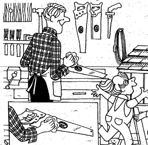
Several handsaws are tools of necessity in any handyman's workshop. Not only can they perform most cutting jobs, but they should do them quickly, easily and accurately. To assure years of performance, wipe the saw after use (inset) with an oily cloth.
