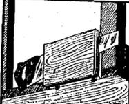
hanging together two 6x10-inch boards and fastening them to the end of your work bench. Glue two pieces of felt or sponge rubber to the inside faces of the boards so that they meet with a slight pressure when the boards are closed and fastened with a screen door hook-and-eye. When the felt is saturated with a light machine oil, you just draw the saw through the oiler to do the job.
